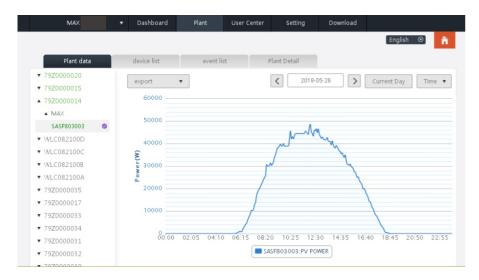
2) By clicking on "power station" and "equipment management" in turn, the real-time data of "data collector", "inverter", "environment monitor", "intelligent meter" and "confluence box" MAX "can be viewed.
