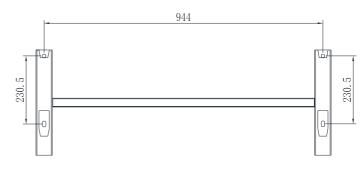
1>Use the wall mount plate as a template drill holes on the wall and put in expansion bolts.
