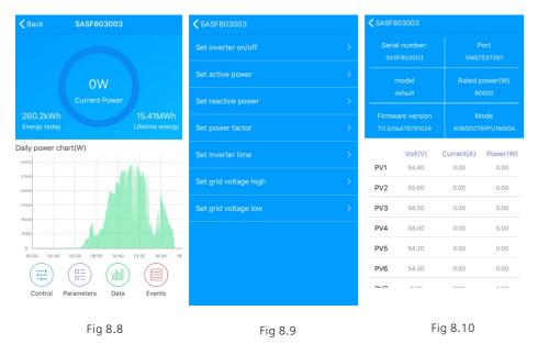
4>Data page: user can see the PV power, voltage, current, R phase power, S phase power, S phase power, T phase power, output power by day, month, year, by finger up cross the screen.
