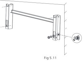
Notice: Do not install inverter unless you have confirmed the wall mount plate has been firmly installed on the wall.
