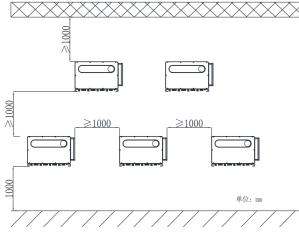
Fig 5.5 D.Do not install inverter into an enclosed space like following drawing.
