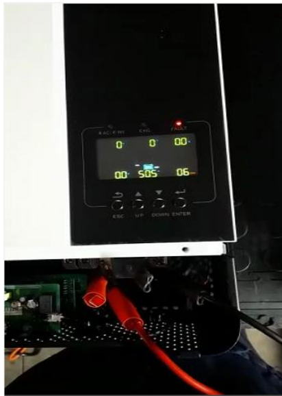
Fig.2 06 fault on inverter display
