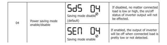
Default value is Sd5, If it is enabled, when the load is lower than 150W, inverter will stop AC output. **Please highlight the point.**
